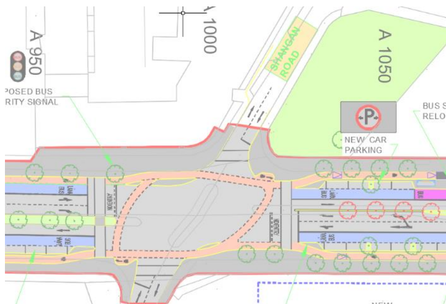
Figure 2-1 Junction Type 1 Proposed Shangan Road Junction
